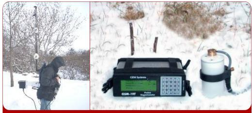
GSM-19TGW Proton Precession console configured with backpack, additional sensor for gradiometer (simultaneous) readings, built-in GPS and VLF EM system
