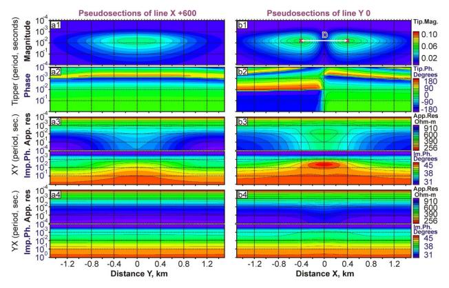
**Figure 3.** Pseudo-sections across Y +600 (a1-4) and X 0 (b1-4) lines. Tipper magnitude (a1,b1); tipper phase (a2,b2), apparent resistivity and impedance phase along XY (a3,b3) and YX (a4,b4) directions.
