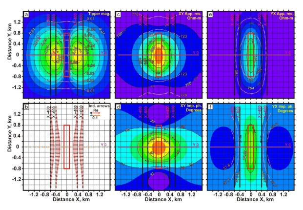
**Figure 1.** AMT-MVP map parameters at 0.008 second (125 Hz). a – tipper magnitude; b – induction arrows in Parkinson convection (pointed to conductor), apparent resistivity (c,e) and impedance phase (d,f) in XY (c,d) and YX (e,f) direction.
