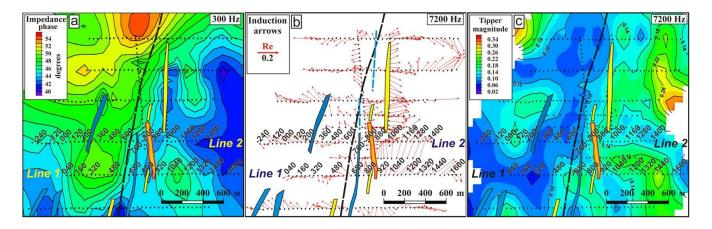
**Figure 2:** Maps of invariant impedance phase at 300 Hz (a), induction arrows (b) and tipper magnitude (c) at 7200 Hz. Orange veins were found by drilling data till 2013, yellow veins are 2014 boreholes results.
