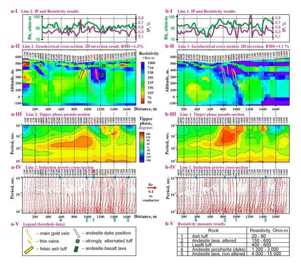
**Figure 3:** AMP-MVP and IP results comparison along lines 2 (a) and 1 (b). The blue rectangles on the upper part of induction arrows cross-sections (a,b-IV) are resistive zones.
